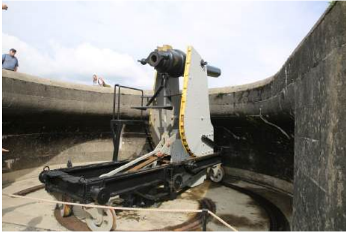
Fig. 2: Crownhill Fort; replica 40 pounder Armstrong RBL (Rifle Breech Loader) on Moncrieff Disappearing Carriage. (Foto: Nick Dougan)
